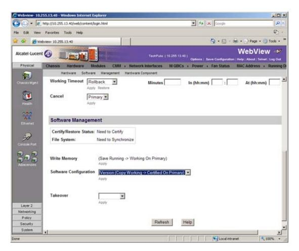
10 In the Software Configuration field, select Copy Working -> Certified on Primary for switches with a single CMM, or Copy Working -> Certified & Synchronize with Secondary for switches with a secondary CMM, then click Apply.
